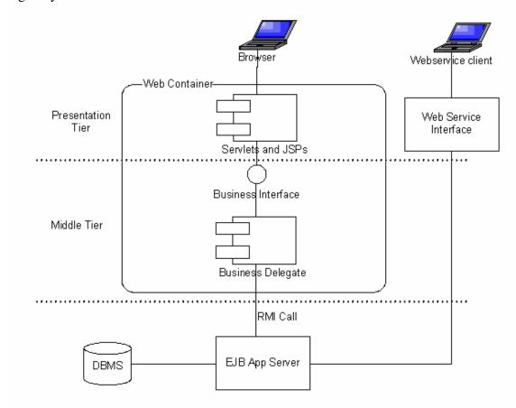
This is a complex architecture with significant overhead. The architecture uses RMI between presentation tier and middle tier. This makes remote invocation a major determinant of performance and design consideration. It forces to minimize number of remote calls.
